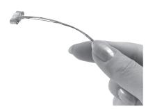
Embedded in resin, the KMP gage measures cure-shrinkage and internal strain. The compact design enables embedment in shaped resins and is suitable for internal stress measurement of products made by combining epoxy resin and metal.
