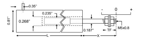
On our unguided LVDTs the armature assembly is a separate component, to make a measurement the user must guide the armature inside the body without touching the sides. Unguided position measurement transducers are appropriate where external guidance is available and give truly non-contact operation
