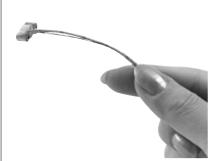
Embedded in resin, the KMP gage measures cure-shrinkage and internal strain. The compact design enables embedment in shaped resins and is suitable for internal stress measurement of products made by combining epoxy resin and metal.
