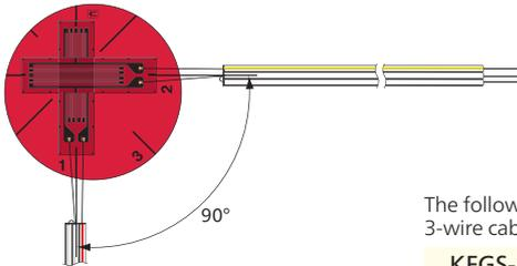
The following model with the lead-wire cable code L1M3S is delivered with a vinyl-coated flat 3-wire cable 1 m long pre-attached.
